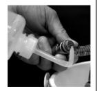
**Note: The syrup system** must be flushed and sanitized weekly. (See PM card SS01 W1.)
