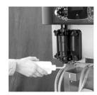
Fill valve cap with sanitizing solution and install. Fill the insulated valve cap with sanitizing solution and install the cap onto the milkshake door spout.
