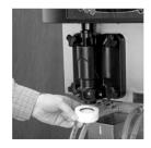
17 Install syrup hole plugs. Raise the retainer pins. Install a syrup hole plug into each syrup port. Lower the retainer pins to secure the syrup hole plugs.
