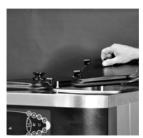
4 Remove, clean, sanitize, and reinstall agitator paddle. Select the calibrate symbol to momentarily stop the agitator paddle from turning.
