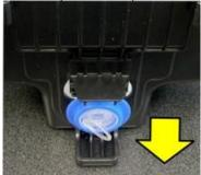
2. Pull the 4 corners of the bag to the 4 corners of the product bin. Lock the clear spout in the keyhole with the guillotine.
