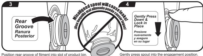
Position rear groove of fitment into slot of product bin. Ensure the fitment is properly snapped into place.
